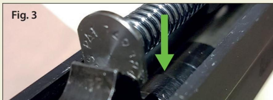
3. Ensure that the DPM system is placed in the correct way, reassemble the slide on the frame and rack the slide several times to confirm that the DPM Recoil system functions unrestricted.
