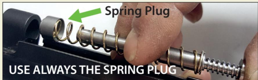
**2. ATTENTION:** Always install the recoil rod base vertically to the barrel correct position. If you place the rod base horizontally, the pistol can't function (Fig. 2, 3)
