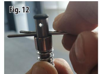
**Step 4:** Insert the Locking Pin to the Assembling/ Disassembling Tool in Option 2, set on a table the Recoil Rod and push to insert complete in to the hole. **Fig 13, 14 & 15**
