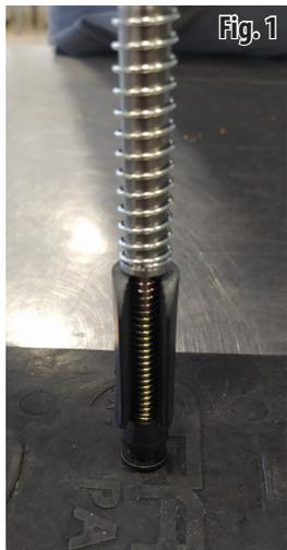
**Step 1:** Adjust the Distance Tool on the Recoil Rod and set the base of the Rod on a non-slippery surface. **Fig. 1**
