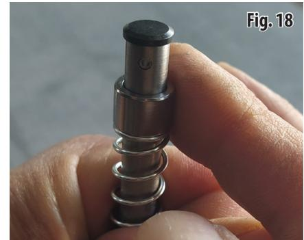
**Make sure that the Safety Pin's edges after the installation are within the Recoil Rod and not outside of it.**
