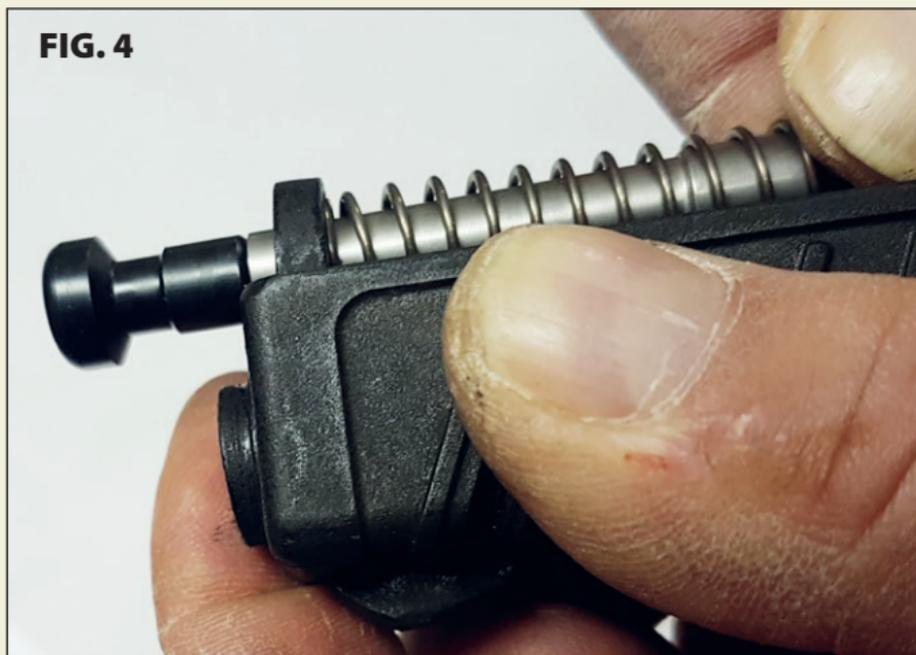
Release the assembling tool and push until the recoil rod passes a little from the slide hole. (FIG. 4)
