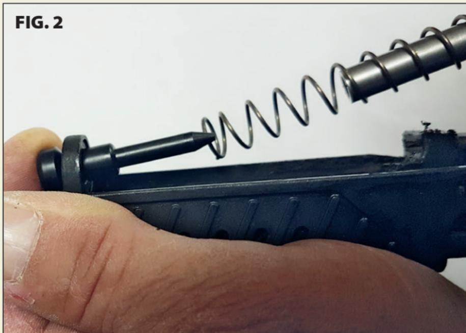
Insert the edge of the spring in the tip of the assembling tool. (FIG. 2)
