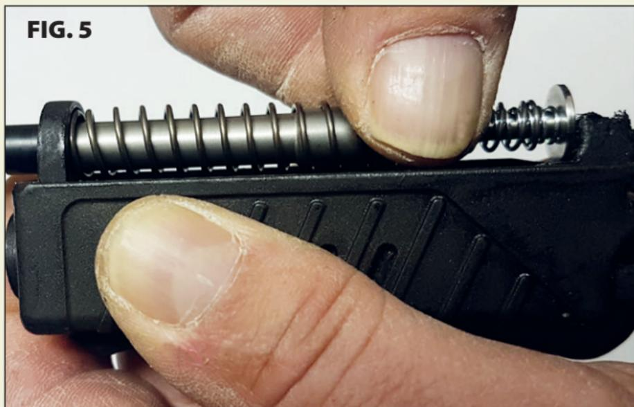
Align the recoil rod and let it sit on the barrel rod position. (FIG. 5)
