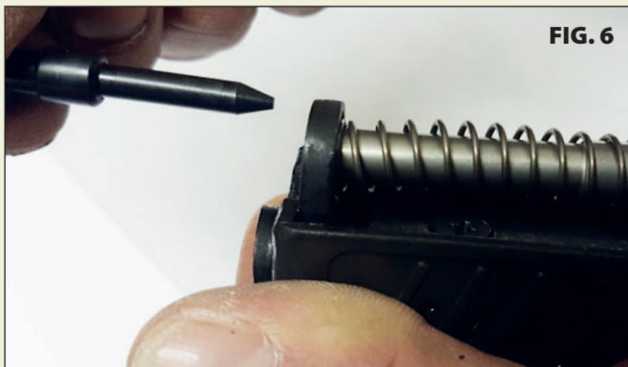
**Remove the Assembling Tool. (FIG. 6)**
