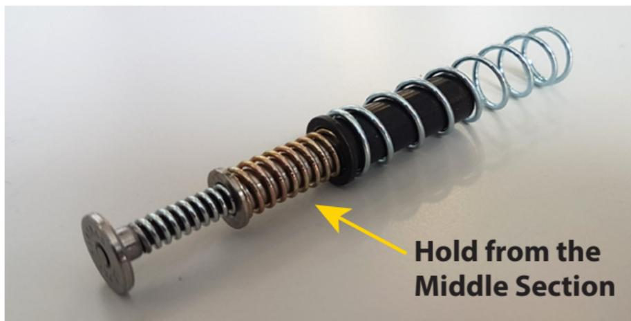
Apply one of the External Springs and hold from the middle section, until the rod passes through the Slide hole for a few millimeters. (Fig. 1 & Fig. 2)
