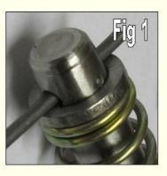
2. Install one spring on the rod and one washer, compress it and insert the safety pin in the small hole of the Rod. (Fig 2). The DPM rod is ready for installation. (Fig1).
