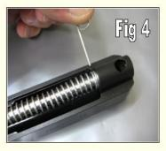
5. Before loading the magazine function (open and close) the slide several times to ensure that the DPM Rod functions unrestricted.
