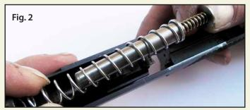
4. Assemble the slide on the frame and rack a few times to confirm that the DPM Recoil Reduction System is installed correctly and the pistol operates unrestricted.
