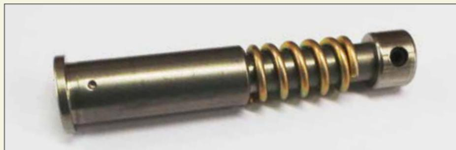
**4.** Insert the main spring to the shotgun tube. In the end of the spring insert also the DPM buffer **FIG 5** and compress completely **FIG 6**. Use the Tool to push inside the DPM buffer until it passes through the second small hole and secure temporarily by using the allen tool. **FIG 7**
