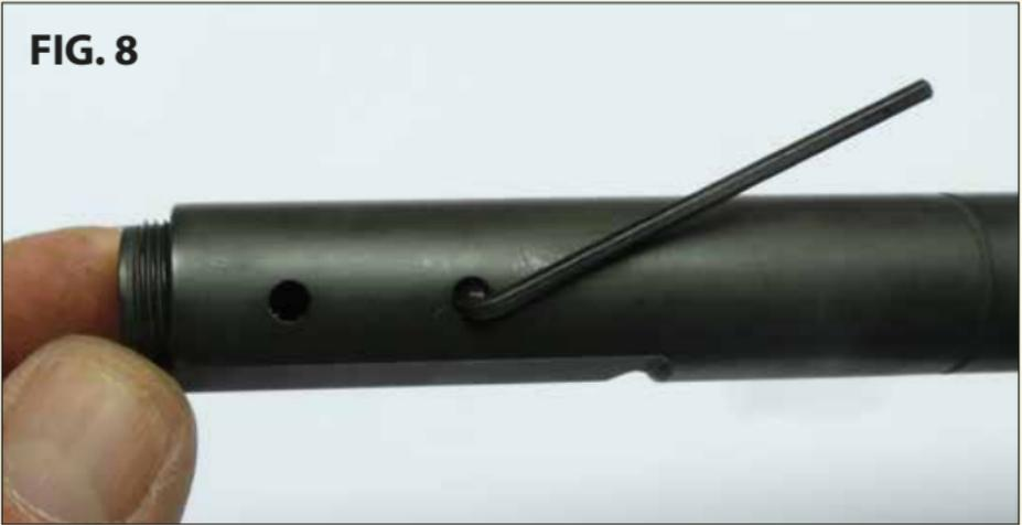
**6.** Attention! Remove the allen tool to release the DPM buffer and the main spring. **FIG 9**
