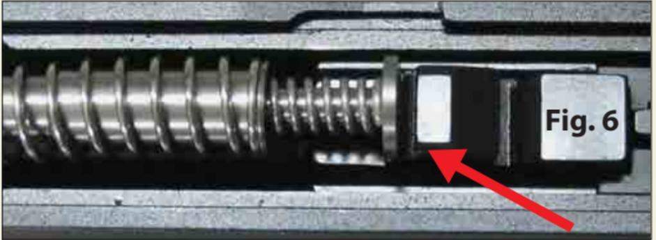
**5.** Assemble the slide on the frame and before loading the magazine, rack the slide several times to ensure that the DPM Rod functions unrestricted.
