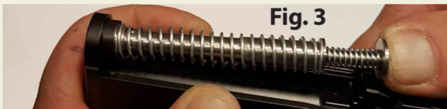
Assemble the pistol and rack the slide a few times to check for any unseen interferences and to ensure that the DPM Recoil System operates unrestricted.
