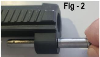
If the big diameter of the DPM Recoil Rod can inserted to the spring house hole ( Fig 3 ),
