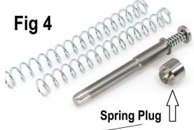
Install one of the external springs on the recoil rod and to the other end of the spring the spring plug and apply to the slide (Fig 5), according to the general installation instructions.
